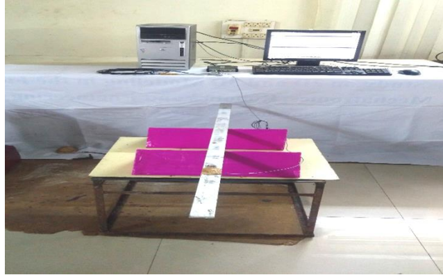
Figure 3. Experimental setup of a free-free aluminum beam
