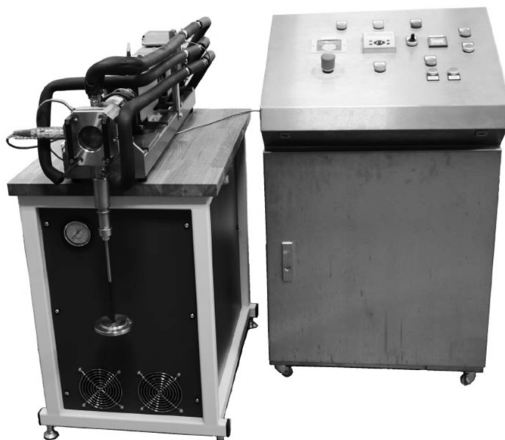
Fig. 4. View of the T-27 apparatus for testing friction and wear of materials in foil-roller combination Rys. 4. Widok aparatu T-27 do badania tarcia i zużycia materiałów w skojarzeniu folia-rolka
