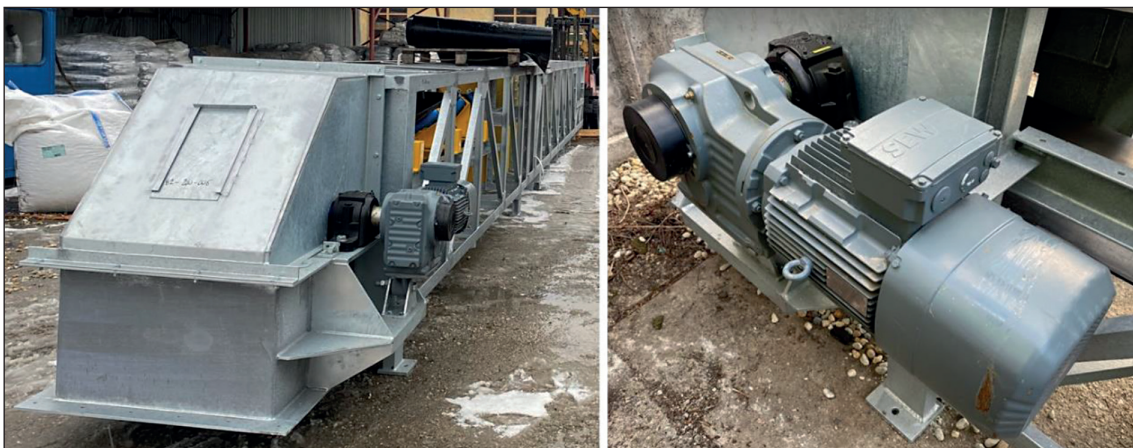
Figure 13. Emptying and drive station
