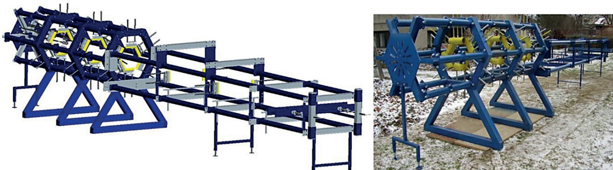
Figure 4. Testing rig for static tests of conveyor belts at TU in Košice [8, 9]
