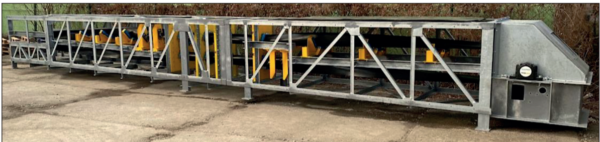
Figure 12. Testing rig for testing conveyor belts and pipe conveyor components
