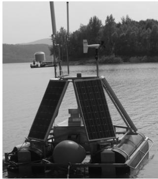
Fig. 4.2. A measurement station for monitoring the quality of drinking water.
