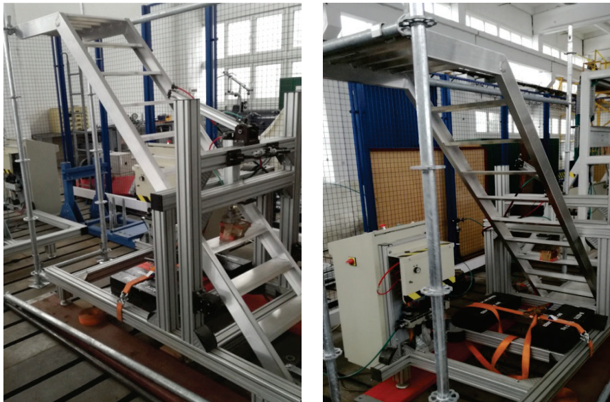
Fig. 8. The set up for fatigue tests
