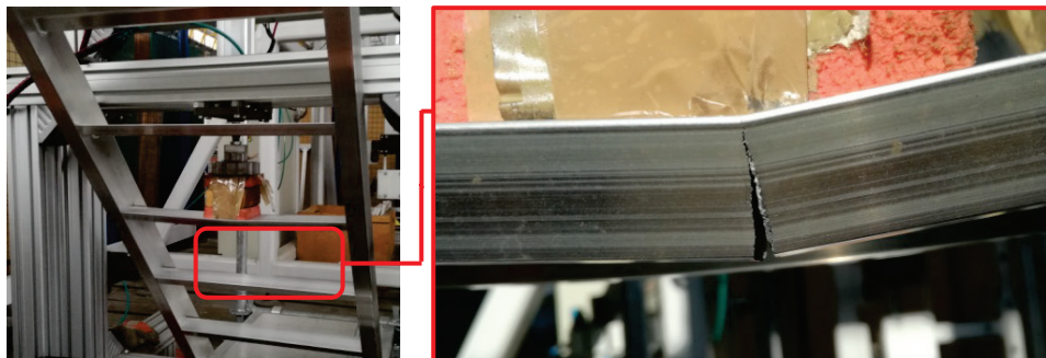
Fig. 10. View of stairs sample after damage due to fatigue load.
