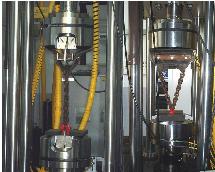
Figure 9. Belt during the lifting test with use of the special fixture
