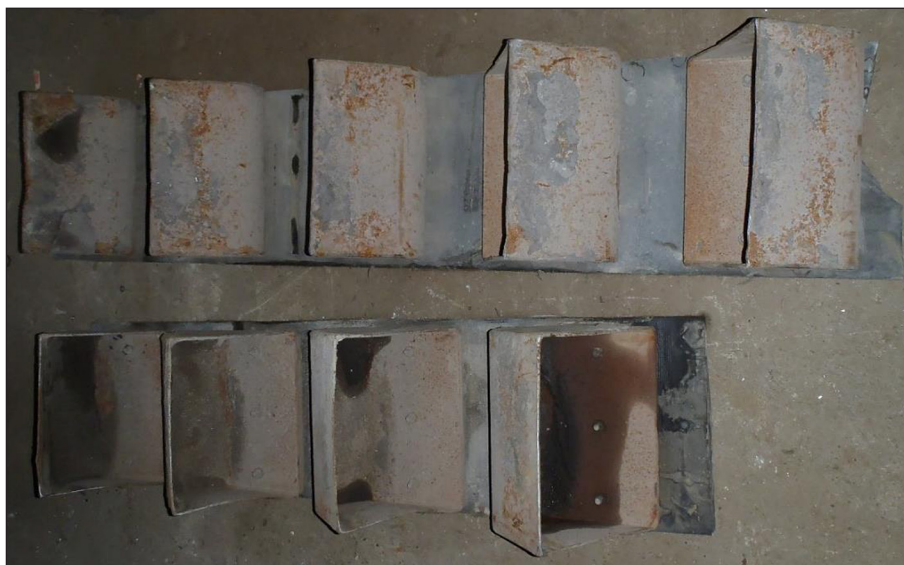
Figure 1. View of two parts of a bucket elevator constituting the sections of a conveyor intended for mechanical testing
