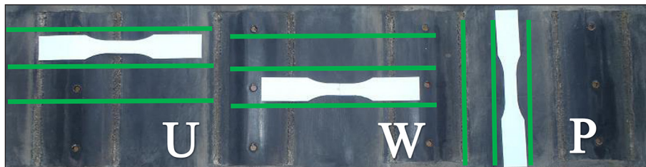
Figure 6. Specimens groups (U, W, P) for strength tests
