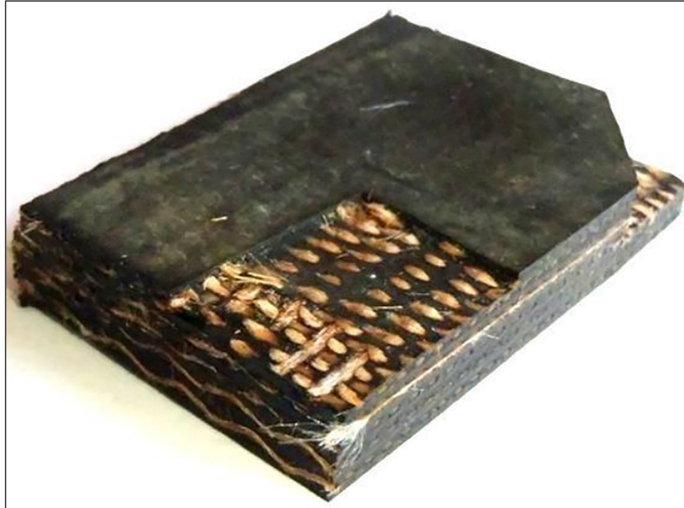
Figure 2. Belt section with selected geometry and weave character
