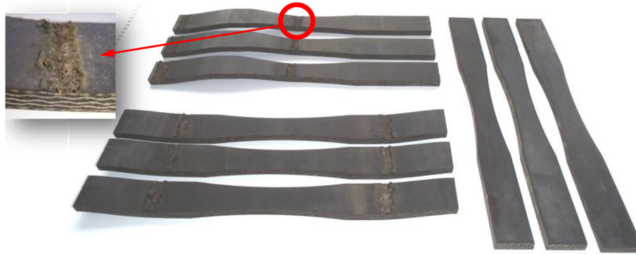
Figure 8. Three groups, specimens designed to perform a tensile test
