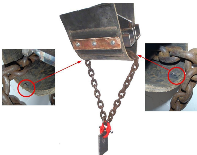
Figure 11. Damage formed in the analyzed belt during the lifting test
