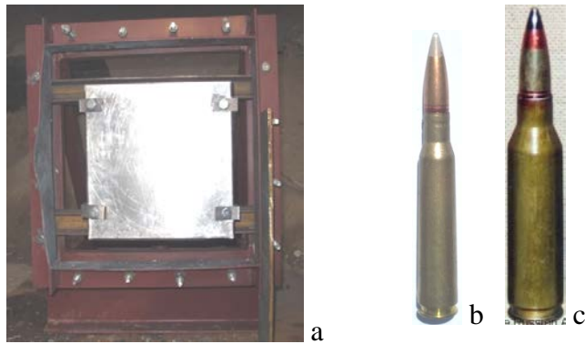
Fig. 5. Test stand and ammunition with the type B-32 projectile: a - stand with an assembled panel, b - 12.7 mm cartridge, c - 14.5 mm cartridge
