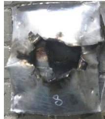
Fig. 7. Specific layers of the panel 4 after firing with the 12.7 mm type B-32 projectile: a - front of the layer 3, b - back of the layer 3, c - front of the layer 4, d - back of the layer 4
