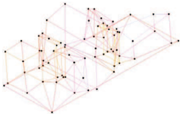
Figure 9. Mode shapes visualization for 49,716 [Hz] frequency for transmission with skew axis for 400rpm [own source]
