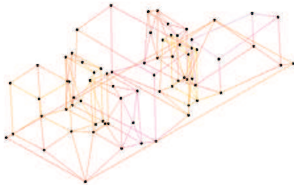
Figure 8. Mode shapes visualization for 384,296 [Hz] frequency for 400rpm [own source]
