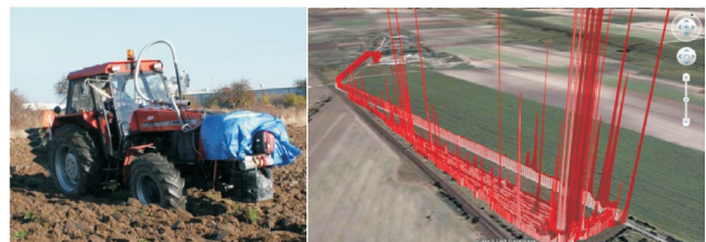
Fig. 9. Farm tractor during the tests under actual conditions of operation and the emission of NO x shown on the tractor route
