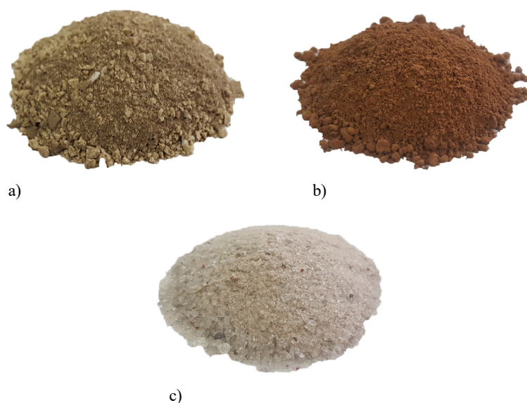
Fig. 1. Shredded: a) utilitarian ceramics waste, b) sanitary ceramics waste, c) CRT glass
