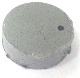
Figure 2. Small hole left on the surface of a PTFE/26.5 wt.% Al composite when laser initiation fails
