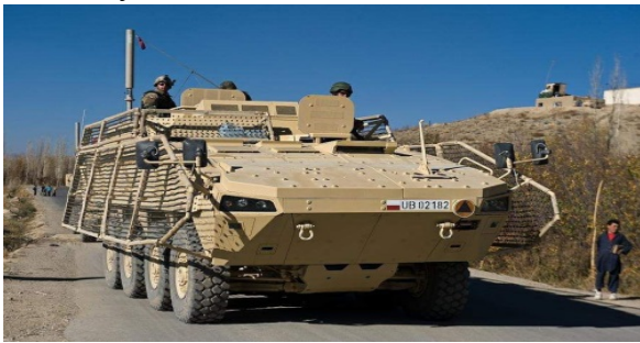
Fig. 4. Example of the use of the cumulative screen on KTO Rosomak vehicle
