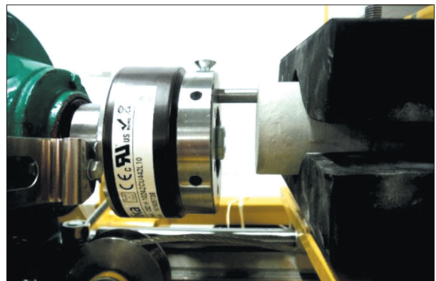
Fig. 2. View of abrasive pair
