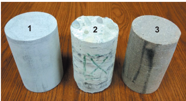
Fig. 3. View of prepared samples for tests: 1 – sandstone, 2 – concrete, 3 – porphyry
