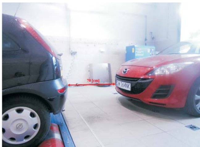
Fig. 1. Setting the vehicles relation to each other during measurement
