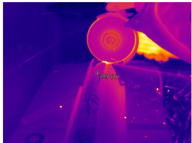
Fig. 1 Mechanical sparks generated by cutting
