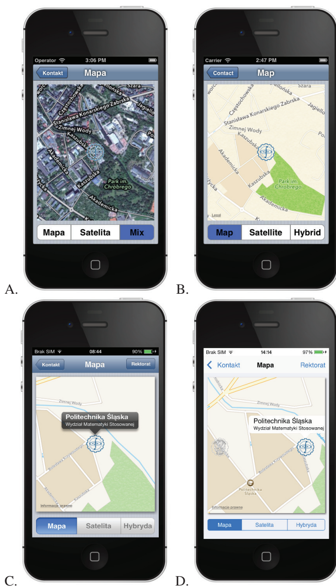
Fig. 3: iOS MkMapView with custom bitmap logo in FireMonkey application A. Polish version of FM1 app, B. English version of FM1 app, C. Polish version, iOS6 (skeumorphic) style, D. Polish version, iOS7 (flat) style.
