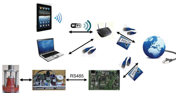
Fig. 8. Connection diagram of the system operating with a public IP address
