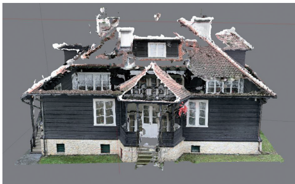
Fig. 6. Solid model developed using Agisoft software app.
