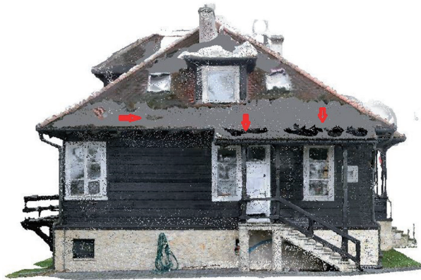
Fig. 3. Model from point cloud with marked faults
