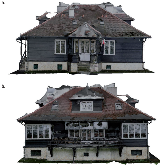
Fig. 5. Solid model of the Estreicher Villa in Kraków developed using ContextCapture software application: a. front view, b. back view
