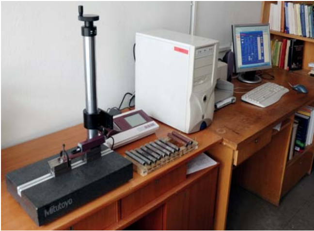
Fig. 2. Mitutoyo SJ-301 Surface Roughness Tester stand, by [self]
