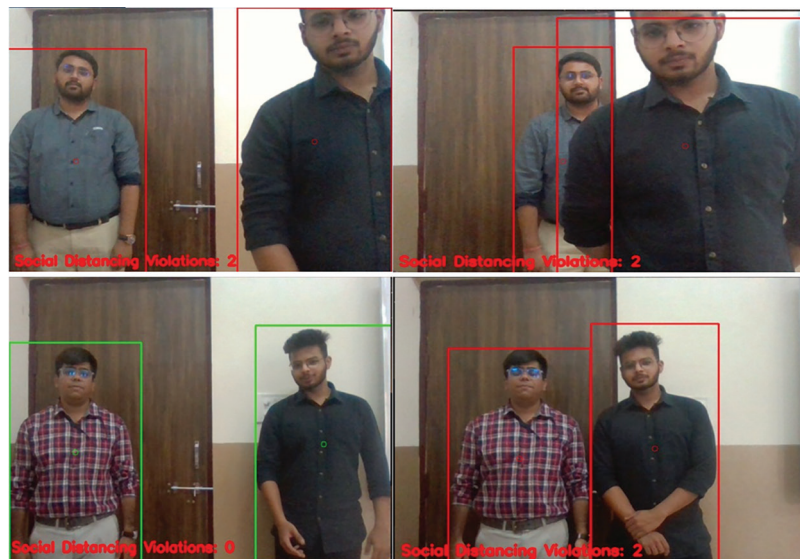
Fig. 10. Social distancing module used at a non-inclined angle
