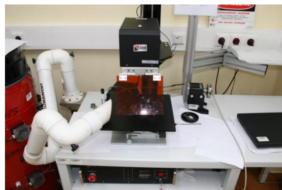
Fig. 3. Experimental setup: fiber Nb:YAG laser
