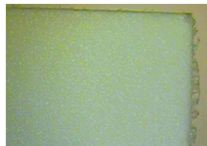
Fig. 2. Burr formation on cut surface
