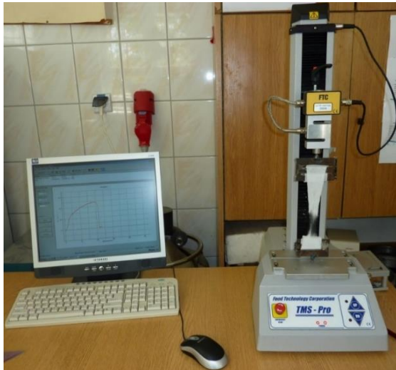
Fig. 6. Photograph of the test stand for force and displacement measurement: Mecmesin TMS PRO with the FTC force sensor, measuring range 0 ÷ 2500 [N] with an accuracy of 0.1 [N]
