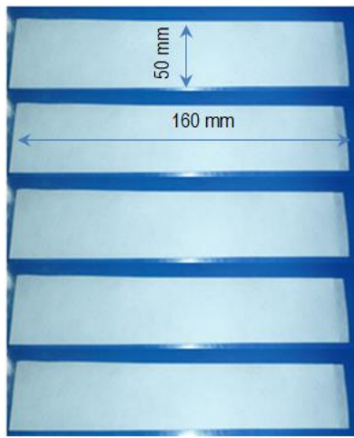
Fig. 5. Example of samples for determination of tensile strength tests
