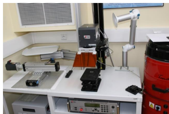
Fig. 4. Experimental setup: diode Nd:YVO 4 laser
