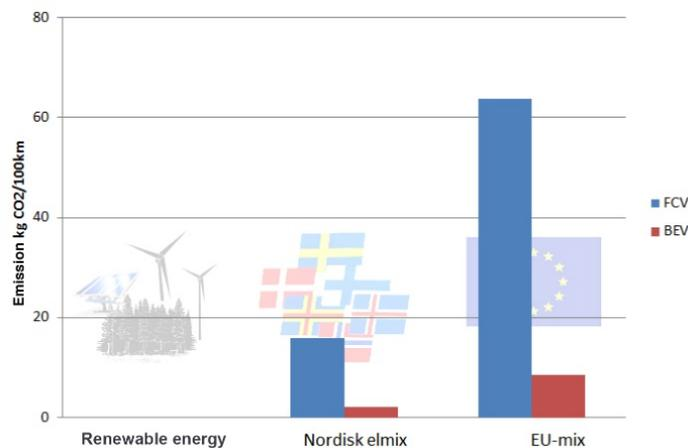
Fig. 1. CO<sub>2</sub> emissions for (BEV) and (FCEV) depending on the origin of the used electrical energy [6]
