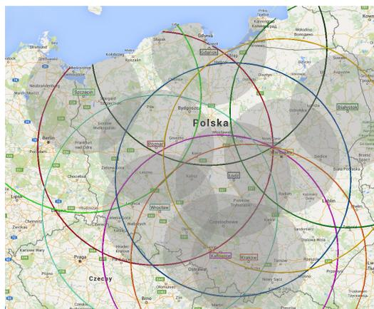
Fig. 2. The movement area of cars using fuel cells based on 9 hydrogen refuelling stations situated on the national TEN-T road network by the 2030 [4], a) when driving in one direction (large circles – to approx. 600 km), b) when driving there and back (small circles – to approx. 300 km)
