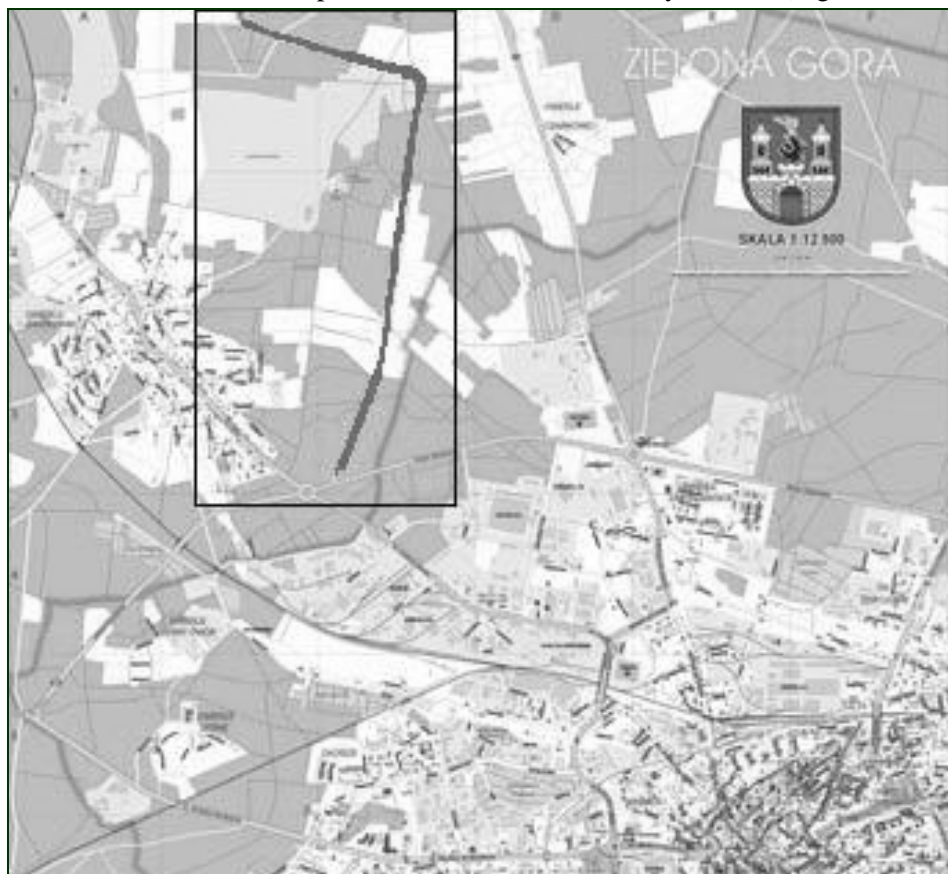
Fig. 2. Plan of Zielona Gora, with marking of the open sewer which carries raw sewage to WWTP
