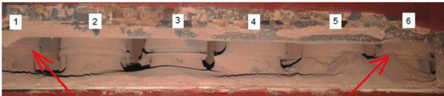
Fig. 19. Dust outlet gaps of individual cyclones, viewed from the multi-cyclone's dust settling chamber, after a period of air filter operation with a dust suction ratio of m_0 = 5\% , during which 2 150 g of dust was fed to the filter: 1, 2, ..., 6 – numbers of consecutive cyclones in a row (the arrows indicate the cyclones whose outlet gaps were blocked with the dust) [8]
