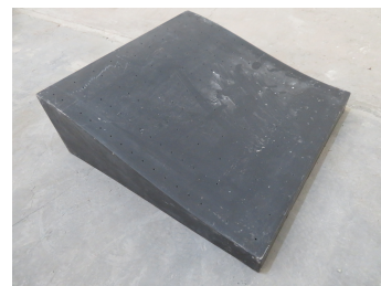
Fig. 2. Non-flat perforated panel (shape C) of 50 \times 50 \text{ cm} dimension.
