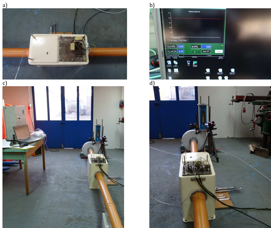
Fig. 1. The measuring station for determining flow resistance by PD - 3A hydrogen incinerator: a) probe connection to pressure measurement; b) indications of the measuring system; c) a complete measuring station for flow resistance determination; d) the examined installation for battery compartment ventilation removed from a submarine, in the background we can see the fan and rotameter for air stream control.
