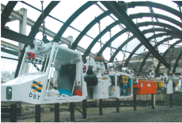
Fig. 9. Battery-driven monorail BZ 45-2-40 of Scharf Company [5]
