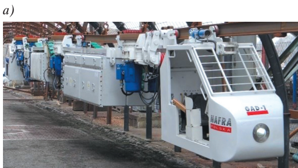
Fig. 12. GAD-1 suspended battery-drive train: a) at manufacturer stand; b) in underground working [8]
