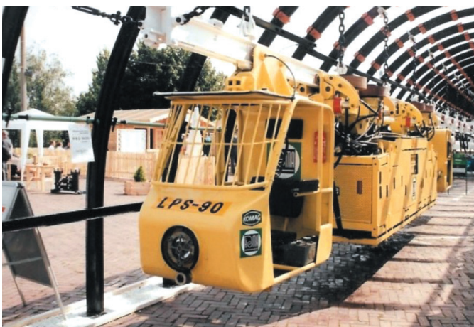
Fig. 5. LPS-90 locomotive (drive train): a) at KATOWICE'95 Fair; b) in underground working [5]
