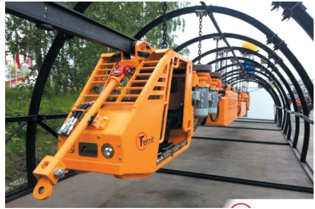
Fig. 10. DLZA 90F battery monorail made by Ferrit [5]
