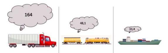
Figure 2. Carbon dioxide emissions released by the different means of transport in gr/tkm (Umweltbundesamt, 2012)
