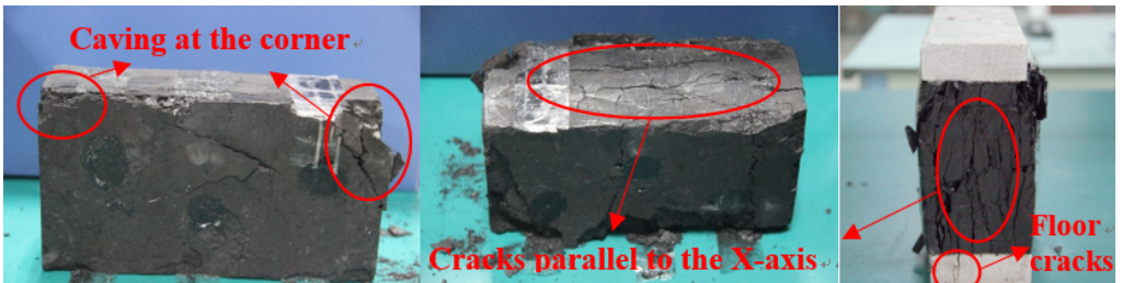
Fig. 11. Failure pictures of test specimens
