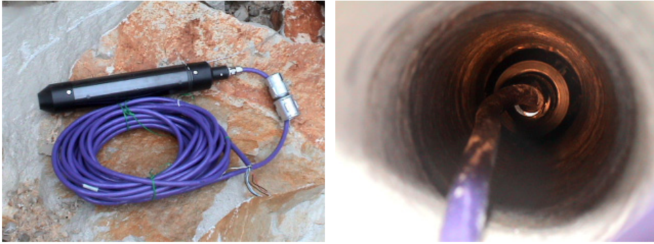
Fig. 7. VW01 Biaxial Stressmeter and its position in the borehole
