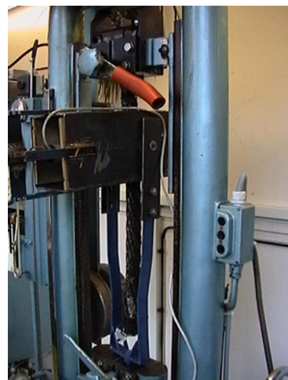
Fig. 5. The shredder and the measuring jig with the rope
