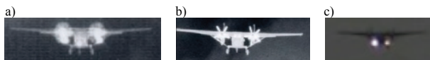
Fig. 10. Exemplary images recorded during observation of BRYZA approaching runway from the distance of 2 km: a) MWIR camera, b) LWIR camera, c) VIS camera
