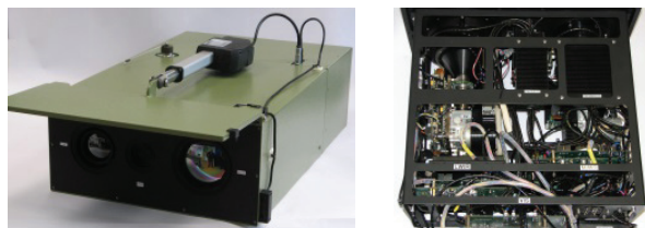
Fig. 3. Photography of Camera Assembly (ZK) comprising two infrared cameras working in MWIR and LWIR spectral range and video camera working in visible spectral range
