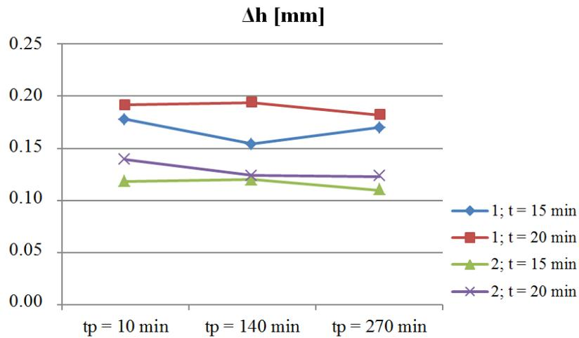
Fig. 5. Dependence between  $\Delta h$  and  $t_p$ , and  $t$  for BC-F400: 1 –  $v = 27$  m/min,  $p = 0.051$  MPa; 2 –  $v = 38$  m/min,  $p = 0.03$  MPa
