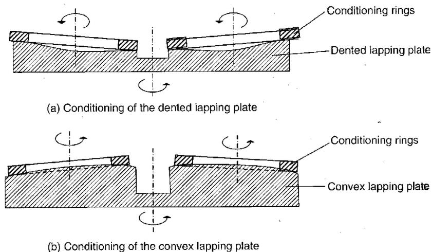
Fig. 1. Conditioning methods of the lapping plate with a conditioning rings [9]
