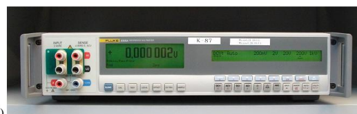
Fig. 5 Selected items in the ITE PREDOM Div. accredited laboratories: a) anechoic chamber with set of antennas applied in EMC tests, b) goniometer for light distribution testing c) spectroradiometer system for tests of photobiological safety of lamps and lamp systems (measuring range 900 – 2200 nm) d) reference multimeter for calibration of electrical test equipment
