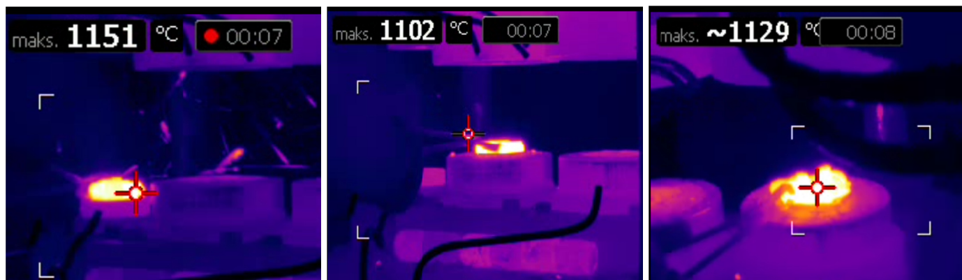
Fig. 2. Stand for forging “adapter”, temperature measurement after flattening operations, initial and finishing forging – temperature of the forging
