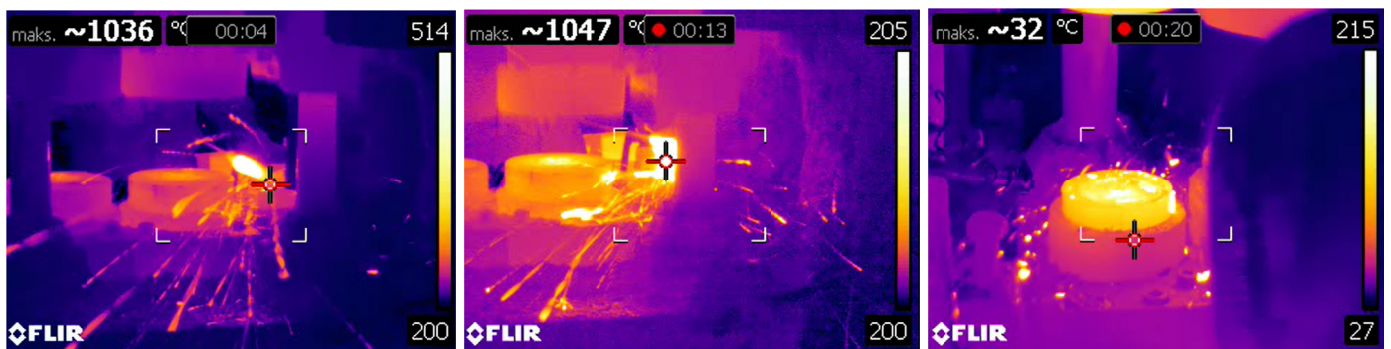
Fig. 9. Visible scale chipping from the forging material and lying on the lower upset dies
