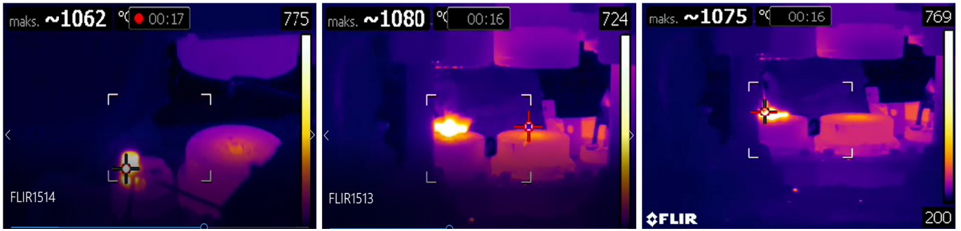
Fig. 4. Stand for forging “yoke” forging, temperature measurement after flattening operations, initial and finishing forging – temperature of the forging
