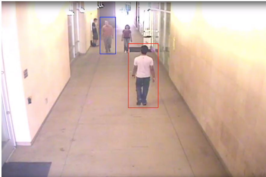
Fig. 5. Recognition of only two people whilst four appeared in the scene. Frame was captured from the database [28].
