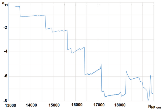
Fig. 4. Coefficient a_{11} of the linear dynamic model calculated by the base thermodynamic model versus operation mode.
