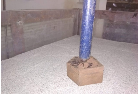
Fig. 2. Placement of skirted irregular pentagonal footing on the sand bed
