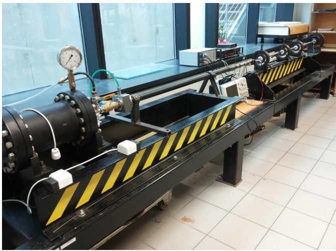
Fig. 5. View of the of the Split-Hopkinson Pressure Bar device used in the research. Projectile launching device including the pressurized gas chamber is visible at far left
