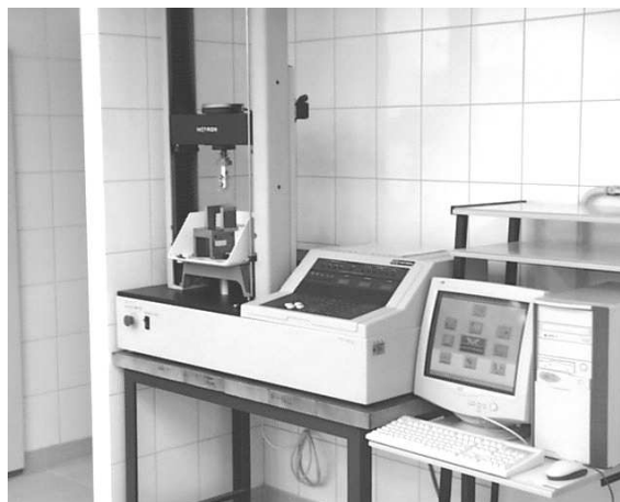
Rys. 2 Stanowisko badawcze do pomiaru tekstury (Instron 4301) Fig. 2. Testing stand to measuring the texture of fruits' gels
