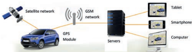
Fig. 1. Diagram of the operation of a vehicle location system [5]
