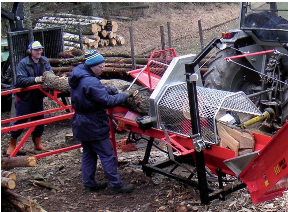
Figure 2. Factory-made firewood harvester with protective cover over cleaving zone. Notes. Photography: Courtesy of Bala Agri AB.
