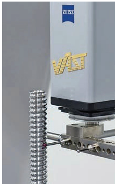
Fig. 5. Racks are allowed to deviate from their ideal roundness by no more than five micrometers, 10 micrometers in diameter and only 0.1 micrometer in surface roughness
