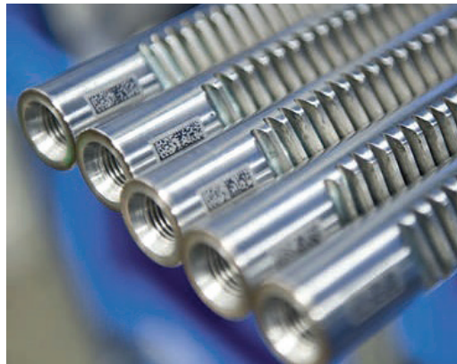
Fig. 3. One of the key parts of an electronic power steering system with a belt transmission is the rack, positioned horizontally between the front wheels
