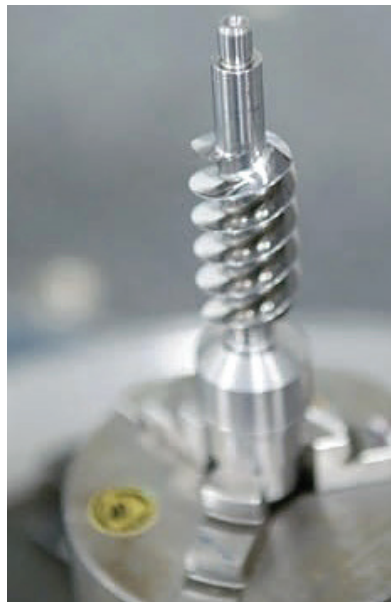
Fig. 7. Worm shaft as a component of the gearbox. Worm gears are used when the gear speed reductions are needed
