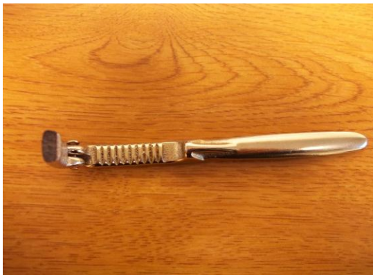
Fig. 1. Fractured gray cast iron nut cracker demonstrating a gray fracture surface
