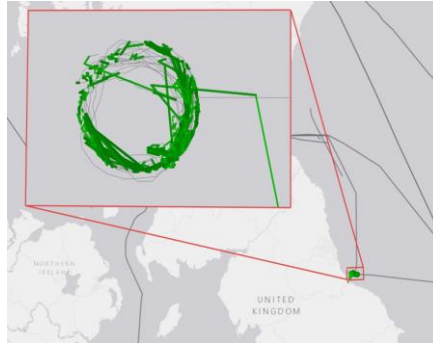
Fig. 15. Example of an angle anomaly (L4) — trajectory of a vessel travelling in small circles
