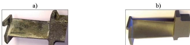
Fig. 5. Low-pressure turbine blade made of Ti-47Al-2W-0.5Si alloy after casting, knockout of the ceramic mould, cutting off the riser (a) and surface cleaning (b)
