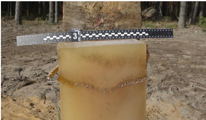
Fig. 4. Damage after a linear charge explosion at a distance of 5 cm
