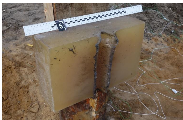
Fig. 6. Damage after a linear charge explosion at a distance of 0 cm
