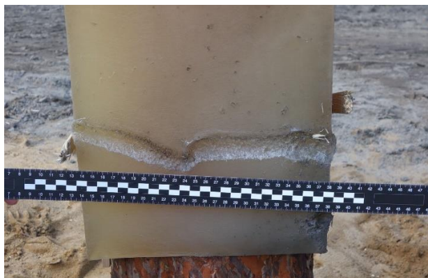
Fig. 5. Damage after a linear charge explosion at a distance of 2.5 cm
