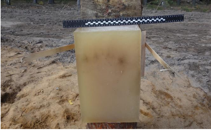
Fig. 2. No damage (sooting only) following an explosion at a distance of 20 cm
