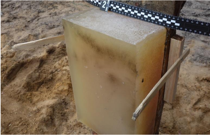
Fig. 3. No damage (sooting only) following an explosion at a distance of 10 cm
