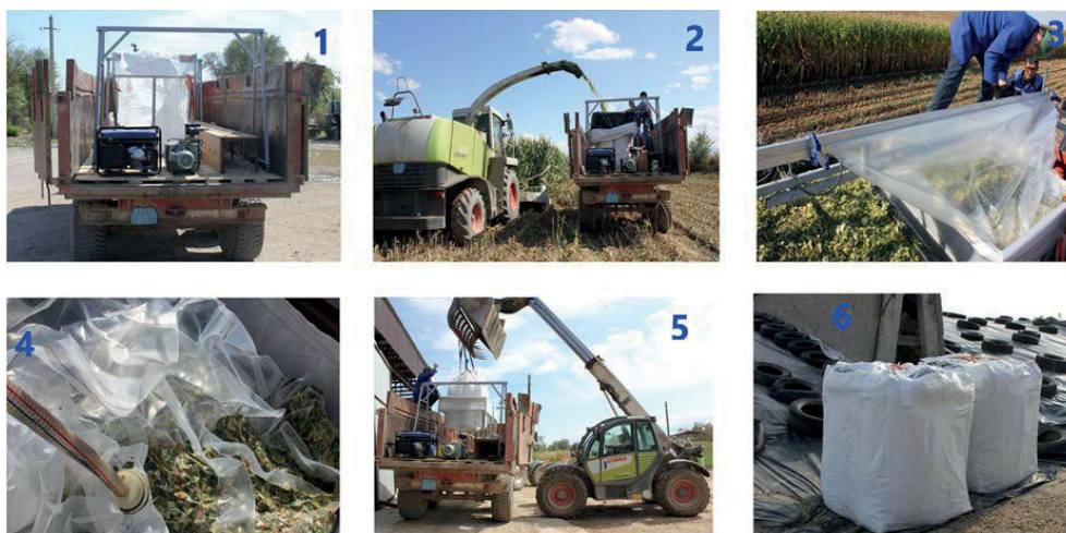
Photo 2. The fragments of of the vacuum silage process in flexible containers on tractor trailer: 1) silage vacuuming on the trailer, 2) converted trailer equipped with the ensiling system, 2) loading of shredded green mass from the forage harvester, 3) sealing of the container by continuous heat sealers, 4) vacuuming, 5) reloading of containers, 6) stacking behind vacuumed containers (phot.: Ye. Zhumagaliyev)
