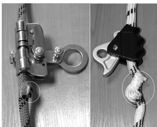
Fig. 2. Examples of damage to flexible anchor line
