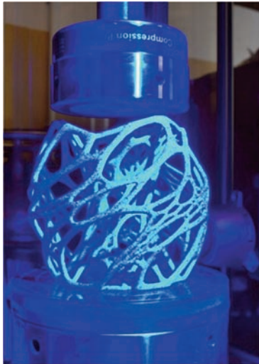
Fig. 4. The three-dimensional bionic structure with applied of the stochastic intensity pattern on the walls
